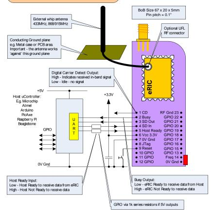
1/4 Wave Whip Antenna 16.4 cms for 433 MHz
