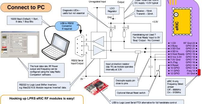
Using an eRIC Breakout Board (BoB) the surface mount castellated eRIC connections are brought out to more convenient 0.1" pitch pins that can be plugged into any prototyping breadboard.
